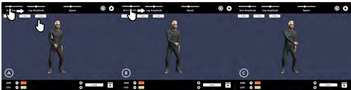
Fig. 6. Motion amplitude adjustment (upper arm used for illustration). Select the desired axis and drag the button of the slider bar of the “Arm Amplitude” to the right. This will increase the range of motion of the arm region. Dragging to the left reduces the motion.
