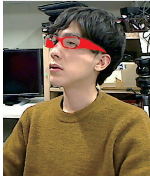
Figure 6: Limitations of our system. In the case that the head pose estimation fails, the virtual eyeglasses and skin texture patch will be misaligned.
