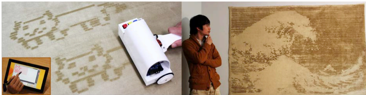
Figure 1: A user draws pattern on a tablet and the device draws the pattern on the carpet (left). The device can draw large images (right).
