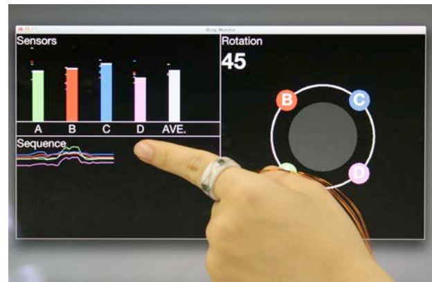
Figure 1: iRing senses finger gestures. Bending, pressure, and rotation are shown on the visualizer.
