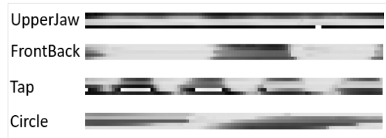
Figure 8. Examples of Grayscale image generated from temporal transition of sensor values of our device for each gesture.
