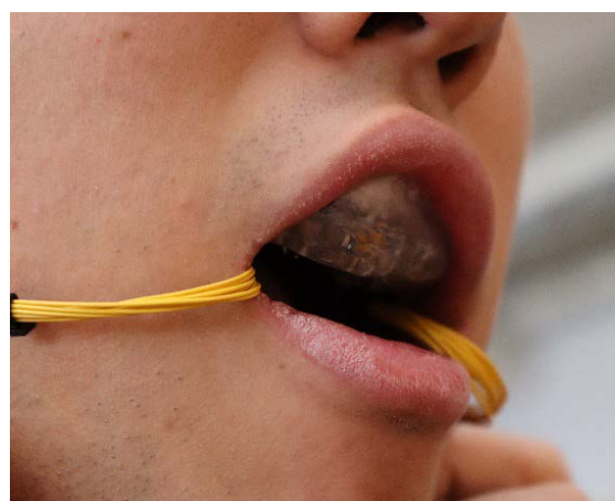
Figure1. Overview of mouthpiece-type sensor that detects tongue motion by photo-reflective sensors
