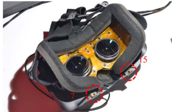
Figure 8: Interior of the HMD. The circuit board is connected via USB port
