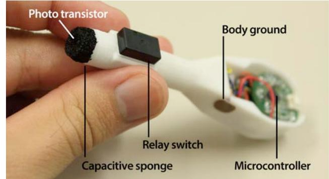
Figure 5. Hardware design of stylus.
