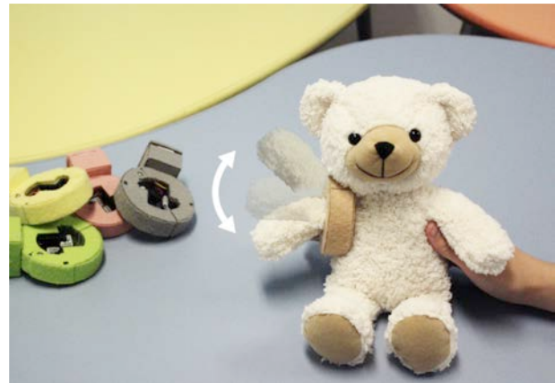
Figure 1. PINOKY attached to the right arm of plush toy, enabling the arm to be moved.
