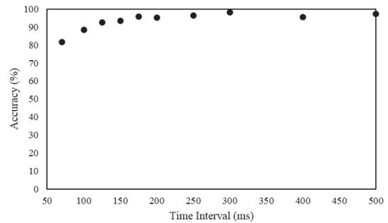
Fig. 7 Relationship between sweeping time interval and accuracy of position detection.
