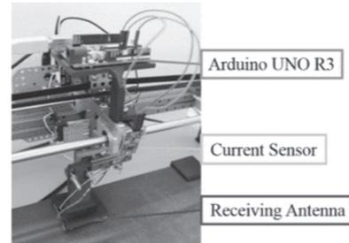
Fig. 3 Power receiving antenna of automatic electrical field mapping system.
