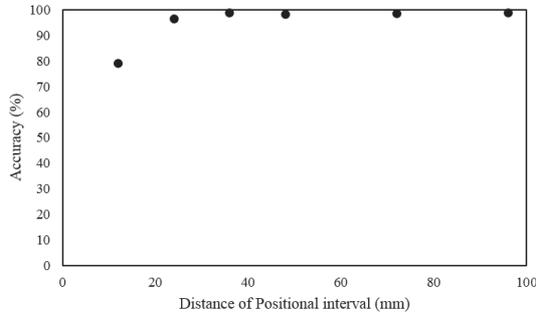
Fig. 9 Relationship between resolution of learning position and position-detection accuracy.
