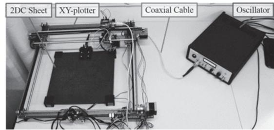
Fig. 2 Automatic electrical field mapping system.
