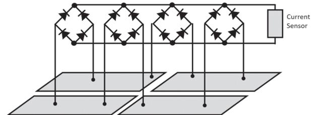
Fig. 4 The rectifier circuit of a receiving antenna with a current sensor.
