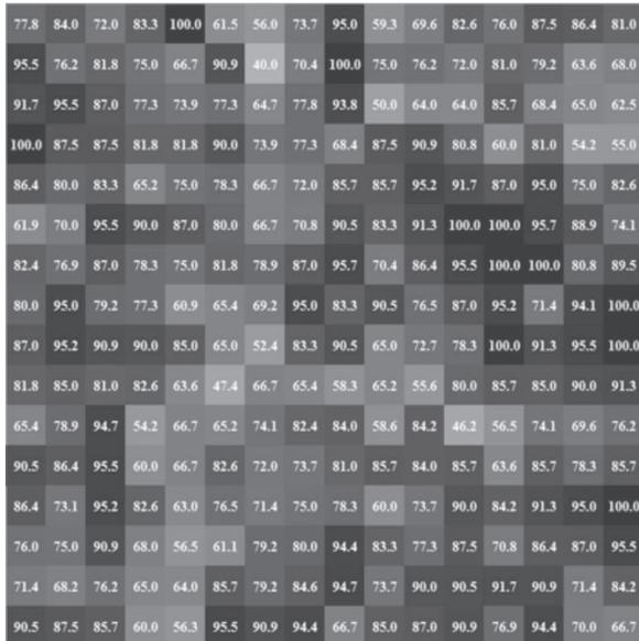
Fig. 10 Position-detection accuracy of each point when moving antenna at 12 mm intervals.
