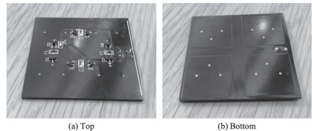
Fig. 5 A receiving antenna, which size is 47 mm × 47 mm.
