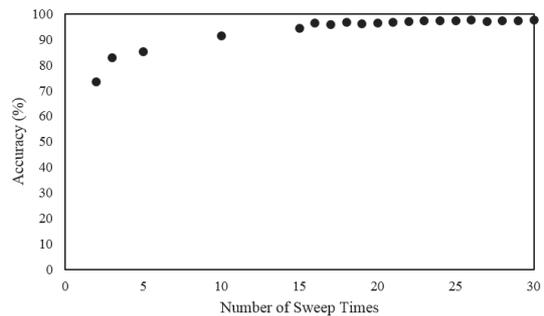
Fig. 8 Relationship between position-detection accuracy of position detection and amount of learning data.
