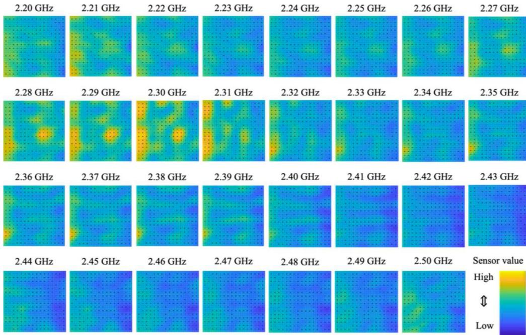
Fig. 6 State of electric field map acquired when manipulating frequency of electromagnetic waves output from transmitter at intervals of 0.01 GHz. Total of 31 electric field maps were generated.
