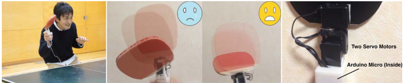
Figure 1: Left: The avatar expresses the intention of the player (Provocation), Middle: The avatar expresses emotions through the motion, Right: The avatar has embedded servo motors.
