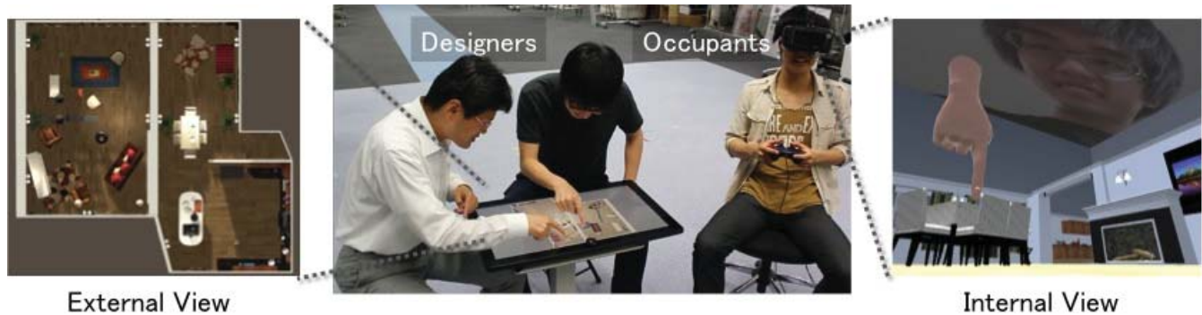
Figure 1: Dollhouse VR interface (center) for asymmetric collaboration with two different views and interaction styles. Top-down view for the designers (left) and immersive view for the occupants (right).
