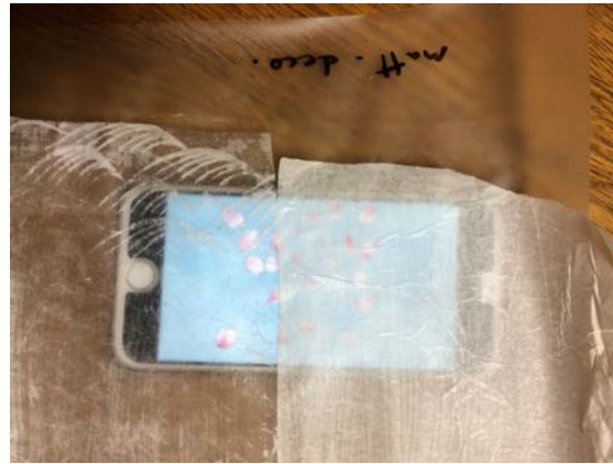
Figure 3: Trying different display panel covers, left the acrylic glass we ended up using.
