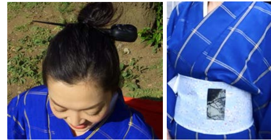
Figure 4: The Kanzashi hair piece with embedded camera adjusted to capture cherry blossom tree crowns on the left, and the camera view on the enhanced obi display on the right.
