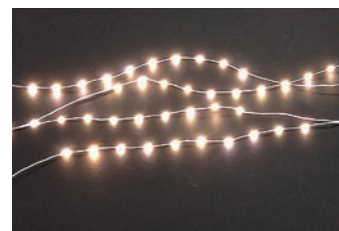
4 LED yarns with applied voltage.
