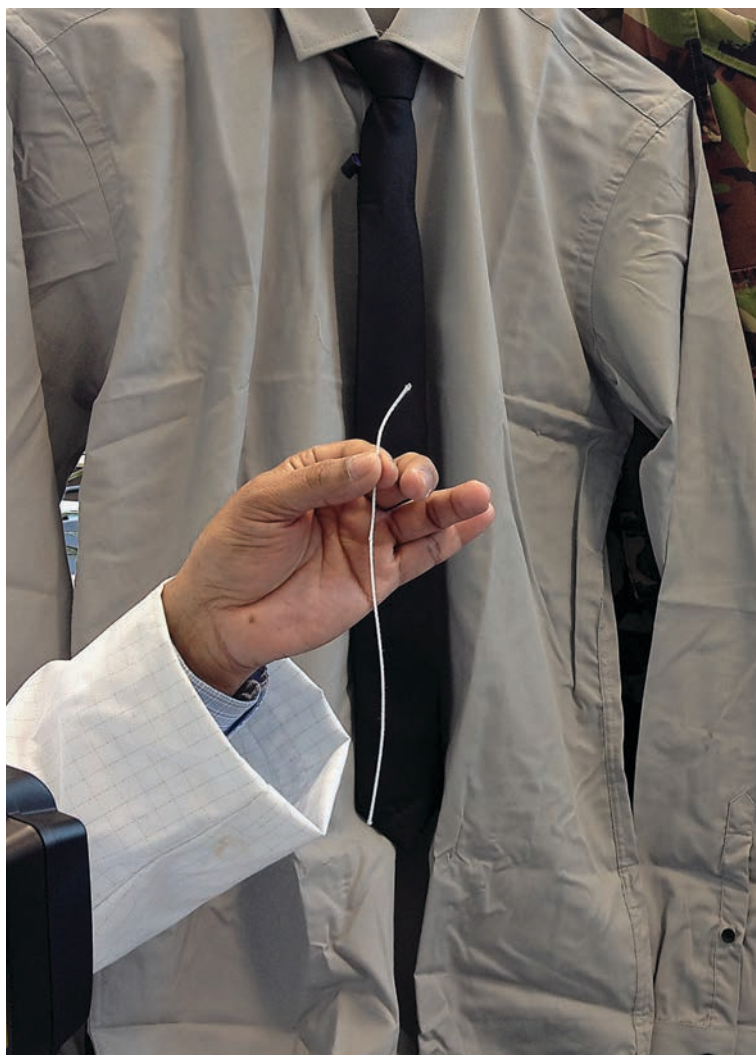
4 RFID yarn alone and integrated into garments.
