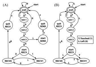
Figure 4. Protocol written in NFA (Nondeterministic Finite Automaton). Diagram represents reception design of (A) reading light on FlashTouch device and (B) sensing touch on mobile application.
