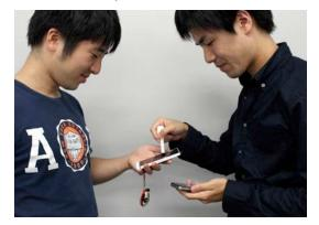
Figure 1. Using the stylus prototype to capture data displayed on a touchscreen.
