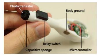
Figure 5. Hardware design of stylus.
